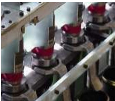
Comando a cintino ogni fuso Single Spindle Tape Drive
